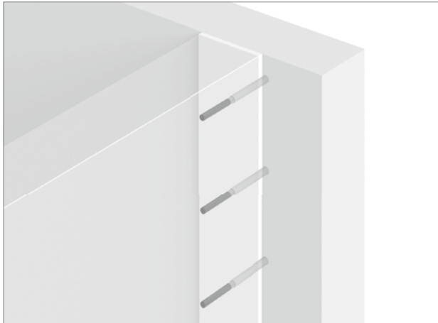
Fig. 11: Schöck Stacon®: wall-wall connection (front-flank)
