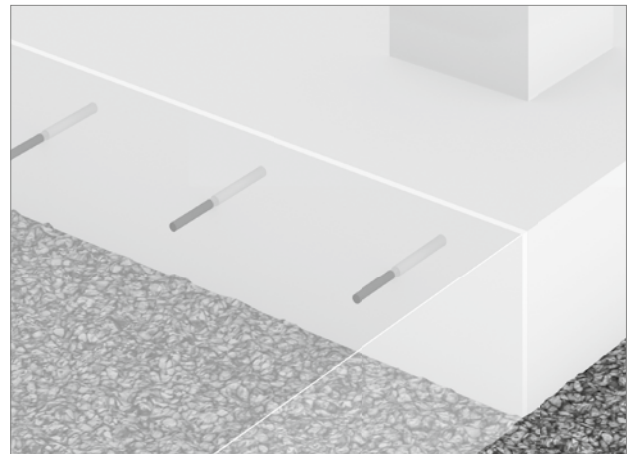
Fig. 14: Schöck Stacon®: Expansion joint in foundation slab
