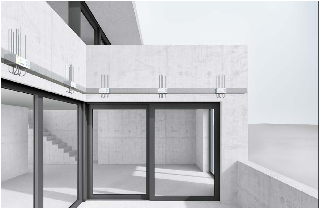
Figure 7: Rendering of an Isokorb® concrete parapet thermal break cast between a concrete roof slab and concrete parapet.
