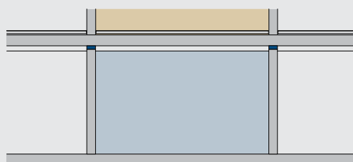
Underground garage / basement: under-slab insulation
